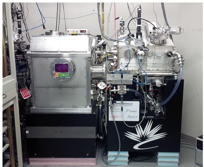
FIG. 1. Photograph of the inboard side of the soft X-ray STXMs at the CLS SM beamline, ambient-STXM (left, upstream) and cryo-STXM (right, downstream).
