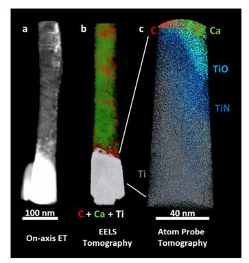
Figure 2: (a) On-axis ET, (b) electron energy loss tomography (EELS ET), (c) APT of the interface of human bone and a Ti dental implant. The TiO and TiN designations are related to detailed analysis of the O and N species from APT spectra [3]. (Adapted from [3]).
