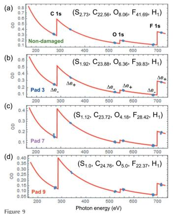
Linear least-squares fitting of the pre- and post-edge intervals (indicated by blue points) of C 1s, O 1s and F 1s edges NEXAFS spectra with respect to the best-found composition of the elemental array **a**. Fitting is presented for four different areas: (a) non-damaged, (b) pad 3, (c) pad 7 and (d) pad 9. The spectra of all 9 pads are presented in Fig. S5. Note the vertical scale differs for each pad.
