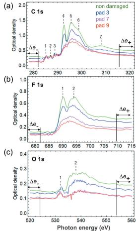
Figure 6 NEXAFS spectra of PFSA(1100) recorded from a 9-pad dose-damage experiment. Panel (a) corresponds to the C 1s edge, (b) to the F 1s edge and (c) to the O 1s edge. The color coding of spectra corresponds to the color of the boxes in Fig. 4(c). The pre-edge and post-edge intervals selected for the elemental component fitting are shown as  $\Delta e_-$  and  $\Delta e_+$ , respectively. The peaks, energies and assignments are presented in Table S4.
