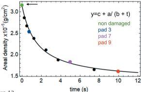
Figure 12 Areal density plotted as a function of exposure time. The colors correspond to Fig. 4(c). The arrow indicates the point corresponded to the non-damaged PFSA(1100) with a targeted elemental composition (S<sub>1</sub>, C<sub>20</sub>, O<sub>5</sub>, F<sub>39</sub>, H<sub>1</sub>), density of 2.0 g mol<sup>-1</sup> and 150 nm thickness. The solid curve is a hyperbolic fit (see Section SI8).
