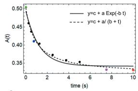
Figure 8 Optical densities A(t) for all pads of the 9-pad damage experiment on PFSA(1100) (Nafion<sup>TM</sup> D521) including the non-damaged area taken at 320 eV (damage energy). The color coding of points corresponds to the color of the boxes in Fig. 4(c). The curves correspond to the linear least-squares fittings according to model 1 (solid) and model 2 (dashed), see Sections SI3.1 and SI3.2.
