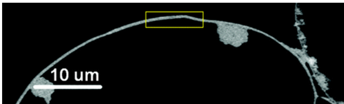
Figure 2.2 STXM overview image (optical density) at 285.2 eV, of PID capsule wall prepared at 50 °C. The yellow rectangle indicates the area where the image sequence for Figure 2.4 was recorded.
