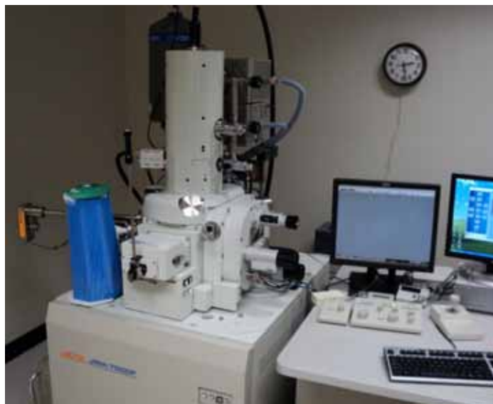
Figure 2.13: Photograph of the JEOL JSM-7000F scanning electron microscope.
