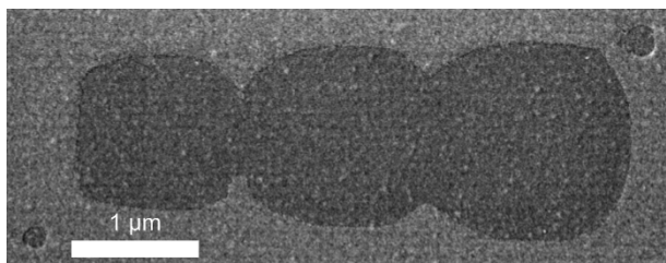
Figure 12.2: Scanning electron micrograph of developed PMMA patterned at 185 eV using 11.0.2.
