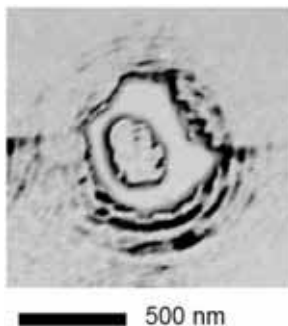
Figure 2. High magnification AFM phase image of the 5000 ms single pixel exposure from the top right corner of figure 1.
